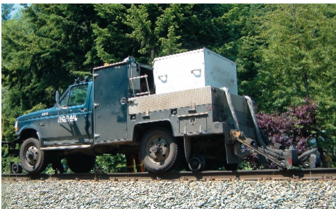
Portec Rail ROAD-RUNNER™ Hi-Rail™ TOR Application System
